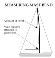
Now it's time to go sailing. Put the boat hard on the wind in at least 10 knots of wind. It's a good idea to have enough crew to handle the boat easily. Use a non-overlapping genoa so that tacking is quick and easy, you'll be tacking a lot while tuning.
