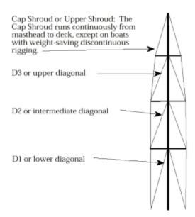
Work down the mast (upper intermediates, lowers, etc.), sighting up the mast for straightness. Relatively speaking, the cap shrouds should be tighter than the intermediates because they are longer and will stretch more under load.
